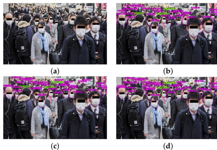
**Figure 9.** (a) Initial image and the classification results of (b) YOLOv3, (c) YOLOv4, and (d) YOLOv4-tiny.
