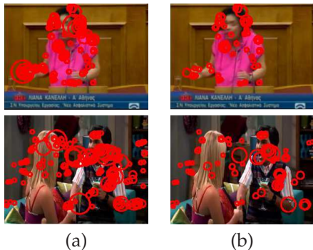
Fig. 2: Representative examples of feature pruning. (a) The original features and (b) the pruned features for the Parliament dataset [19] (top row) and the TV human interaction dataset [21] (bottom row). Feature pruning may reduce the number of features by 29% on average.
