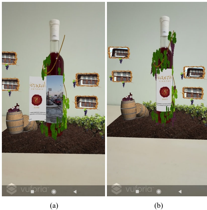
Figure 6 Different instances of the wine ‘live’ label application, (a) the device camera focuses on the bottle label and the ‘virtual door’ opens revealing a hidden video content (b) the ‘virtual door’ closes and the 2D animation of the vine branches progressively appears (see online version for colours)
