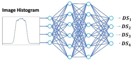
**Figure 1: Schematic description of the neural network approach described in this paper. The input of the NN is a back-scattered electron image histogram and the output is a prediction of the GMM deconvolution success.**
